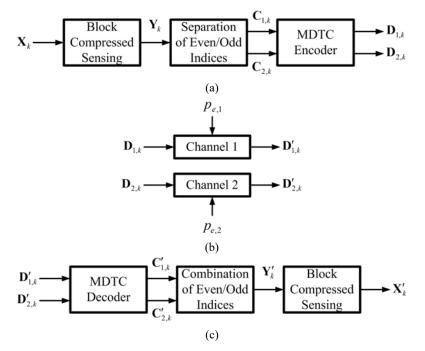
Fig. 1. Block diagrams for transmission with BCS and MDTC.
